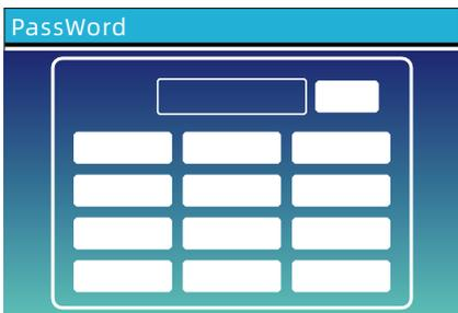
Systemselfchek:After ticking this item, it needs input the password. The default password is 1234. After input the password and then tick "OK"
