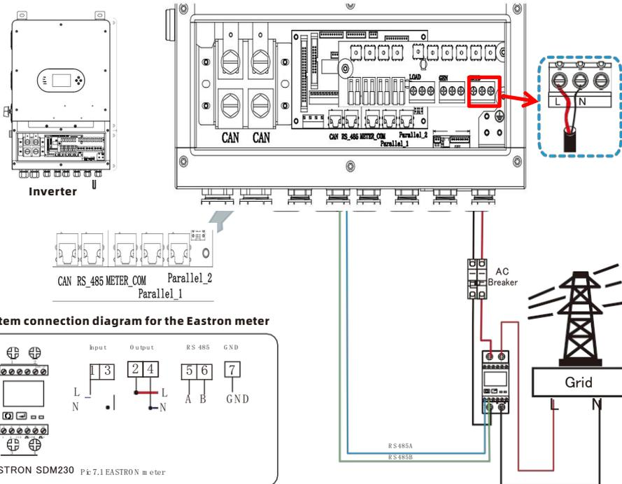
**Note:** In final installation, breaker certified according to IEC 60947-1 and IEC 60947-2 shall be installed with the equipment.
