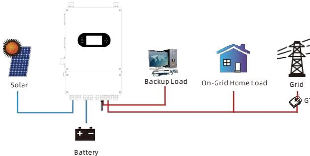
Solar Sell: "Solar sell" is for Zero export to load or Zero export to CT: when this item is active, the surplus energy can be sold back to grid. When it is active, PV Power source priority usage is as follows: load consumption and charge battery and feed into grid.
