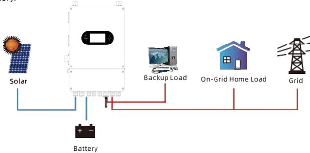
**Zero Export To Load:** Hybrid inverter will only provide power to the backup load connected. The hybrid inverter will neither provide power to the home load nor sell power to grid. The built-in CT will detect power flowing back to the grid and will reduce the power of the inverter only to supply the local load and charge the battery.
