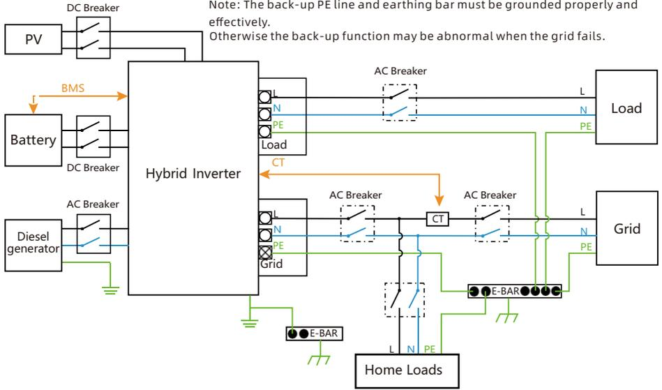
This diagram is an example for application that Neutral connects together with PE in distribution box.
