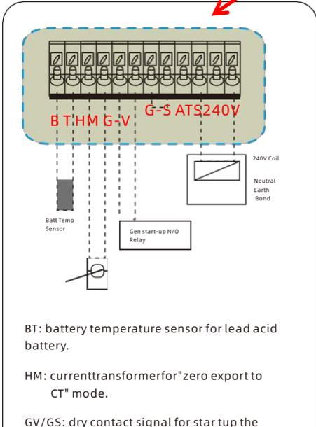
BT: battery temperature sensor for lead acid battery.
