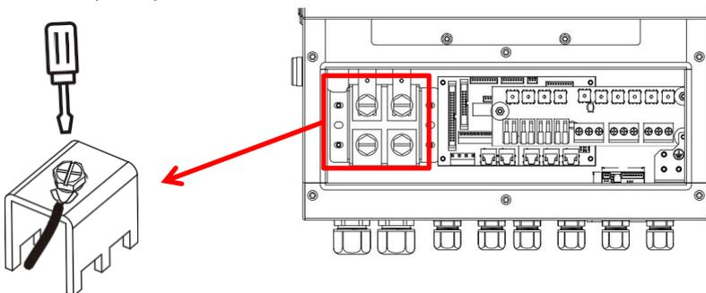
For 5kW/6kW/4.6/8/10/12kW model, battery connector screw size: M10
