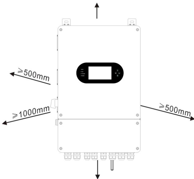
For proper air circulation to dissipate heat, allow a clearance of approx. 50cm to the side and approx. 50cm above and below the unit. And 100cm to the front.
